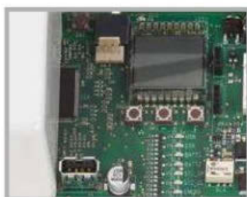
3 USB port for updating and exchanging configuration data
