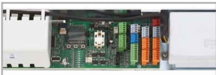
2 Control unit with switching power supply
