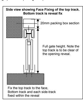
Options Tick Box: With reveal fixing gates, <u>5mm</u> is to be deducted from the width and height of the opening to allow for tolerance. If face fixing 20mm packing box sections are required.
